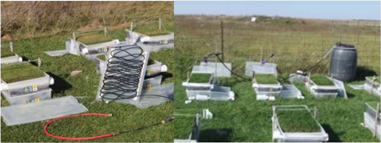
Figure 2: Rain simulations were performed by flowing water through an array of permeable hose (left) so that it dripped down onto the plots. Storm simulations were carried out by pumping water with a well-defined amount of nutrient and sediment from a barrel onto a sheet that directed it to the uphill end of the plot (right).
